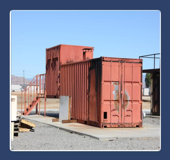
The Phase 1 system (Swedish Flashover Prop) is essentially a laboratory, where fire behavior can be observed from a vantage point three feet below the fire floor. It is designed to help increase knowledge of fire behavior; increase recognition of the warning signs of flashover.
